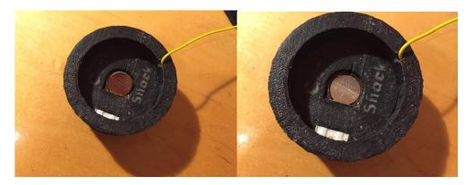
• Now with the boss drilled and fitted to the bus you can place the TX carrier into the boss threading the yellow wire though the 2.5mm hole you have drilled.
