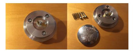
• Now you can unbolt the earth tab, and then replace the allen key bolts and springs.
